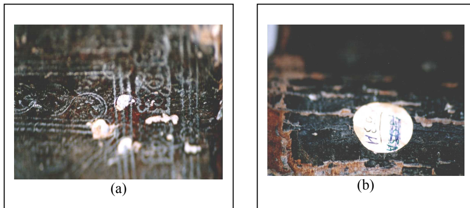
Figure 2. Details of the: (a) physical degradation; (b) chemical degradation.
