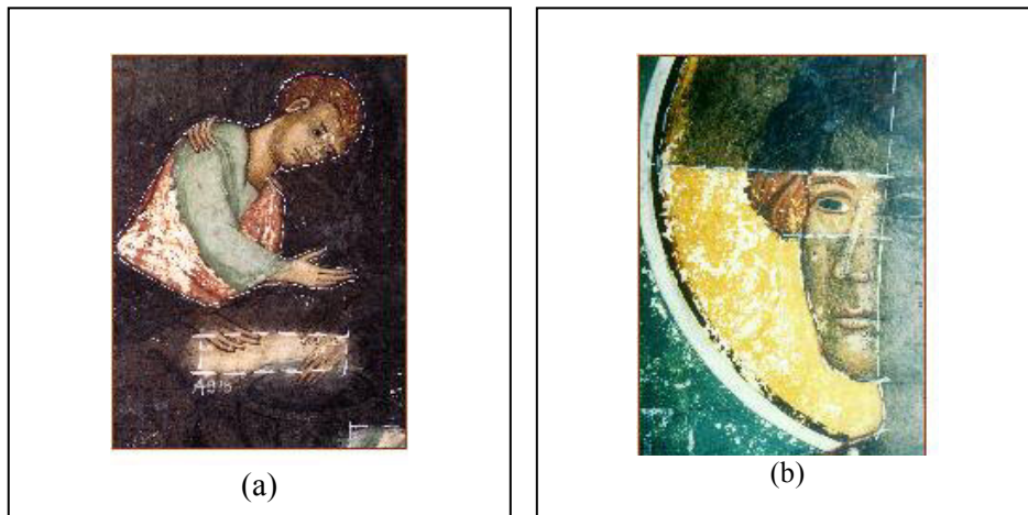
Figure 2. Cleaning tests of the mural paintings: (a) altar; (b) nave, south wall.
