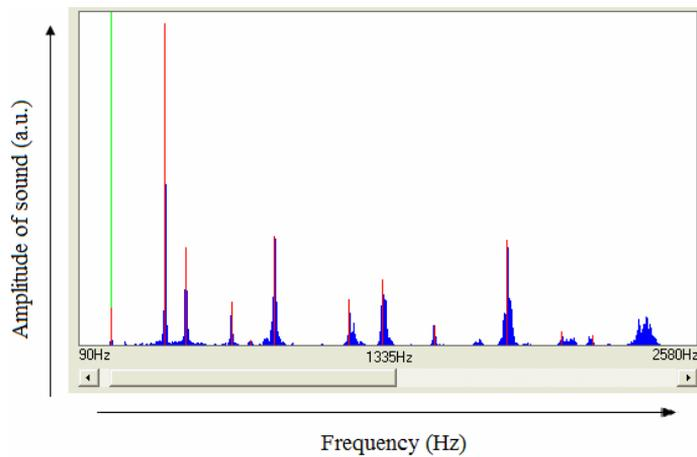
**Figure. 2** Fourier transform of the recorded bells' sound as resulting from the Wavanal program.
