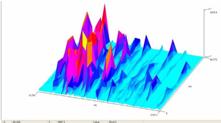
**Figure 15.** 3D time FFT analysis: x-axis: time (s), y-axis: frequency (Hz), z-axis: amplitude, for the witness sound.
