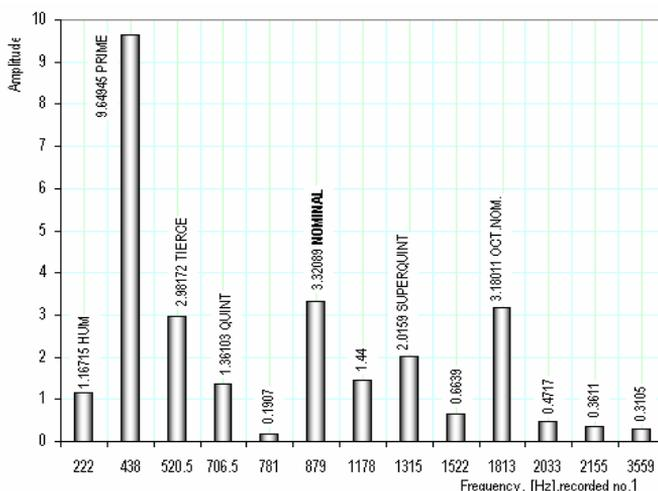
**Figure 4.** Amplitude dependence on frequency for the recorded sound from the ringing bells.
