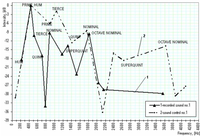
**Figure 9.** Intensity of sounds versus frequency plots for the main partials of the two analyzed sounds.
