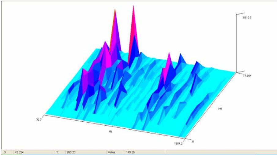
**Figure 14.** 3D time FFT analysis: x-axis: time (s), y-axis: frequency (Hz), z-axis: amplitude, for the recorded sound.
