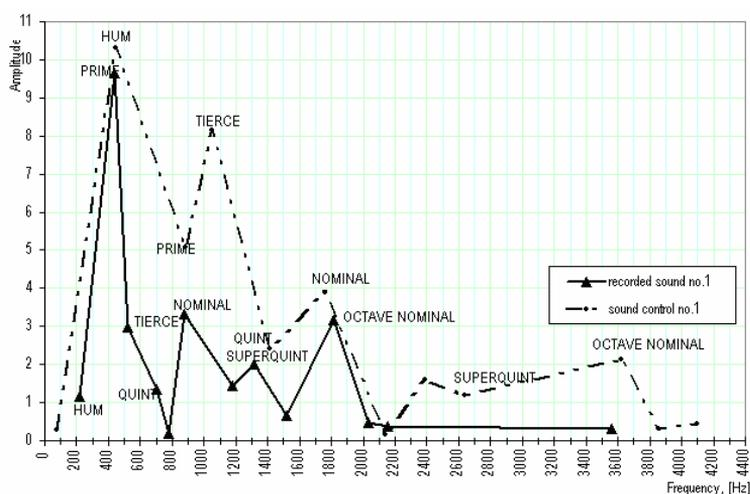
**Figure 8.** Amplitude of sounds versus frequency plots for the main partials of the two analyzed sounds.
