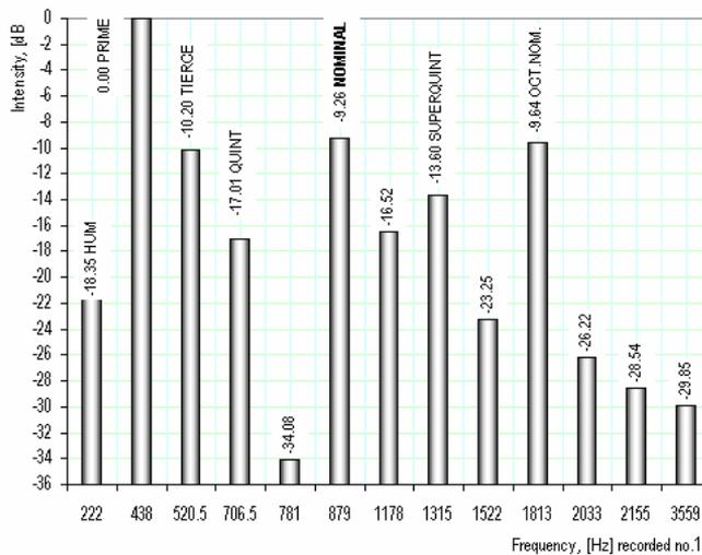
**Figure 6.** Intensity of sound versus frequency for the recorded bells' sound.
