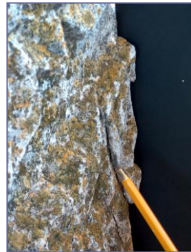
Figure 4. Detachment on contour scaling and deposits of biological colonization
