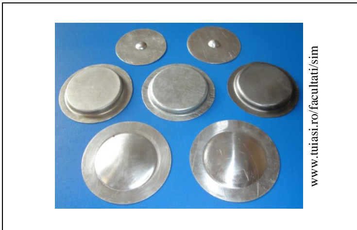
Figure 7. Examples of deep-drawn parts by electromagnetic forming.
