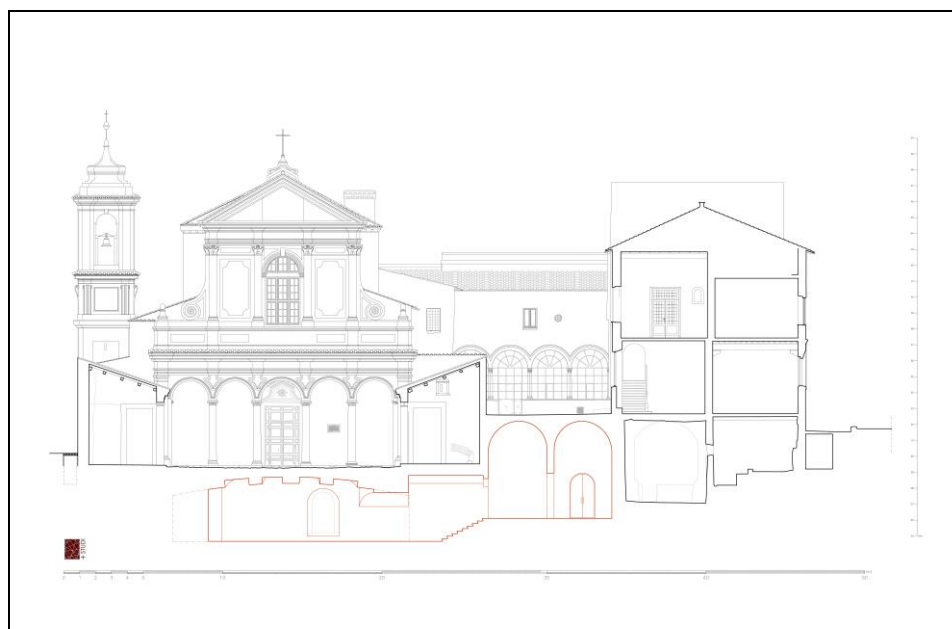
Figure 13. San Clemente ‘final’ project: cross section with the new underground hall (survey by ICR, AZIMUT sas, drawing by R. Cerro and V. Leone).
