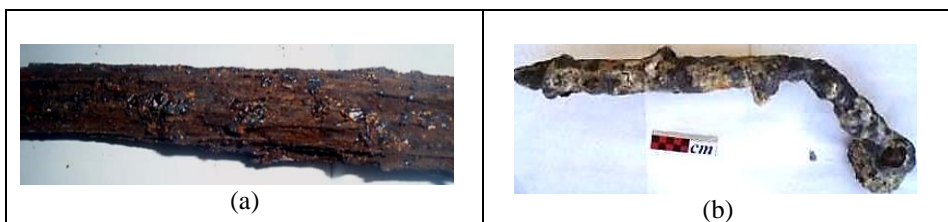
Figure 5. (a) Weeping aspect of marine iron object after excavation for 6 years, (b) Wrought iron object that represents the top part of historical ship.
