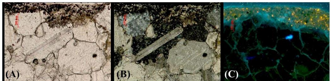
Figure 3. Microphotographs under polarizing microscope of sample CMG1, objective 10x: (A) Parallel polars, (B) crossed polars, (C) UV radiation.
